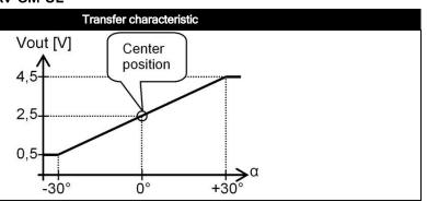
Default 0°: horizontal (round nose upwards), no acceleration applied.
