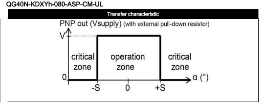
The default 0° position is when the sensor is mounted horizontally (round nose upwards) and no acceleration is applied.
