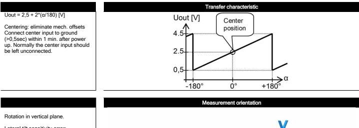
Lateral tilt sensitivity error:  $< \pm 0.03^{\circ}$  lateral tilt (typ.) Max. lateral tilt: 45°
