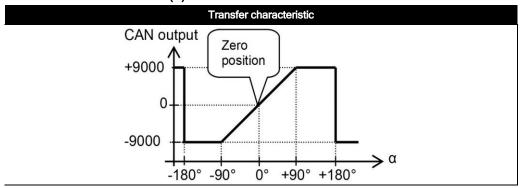
Default 0°: horizontal (label upwards), no acceleration applied. To eliminate mounting offsets the sensor can be centered within ±5° tilt (by the CAN object dictionary)
