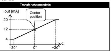
Default 0°: horizontal (round nose upwards), no acceleration applied.
