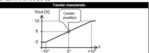
Default 0°: horizontal (label upwards), no acceleration applied.
