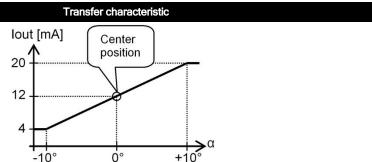
Default 0°: horizontal (label upwards), no acceleration applied.
