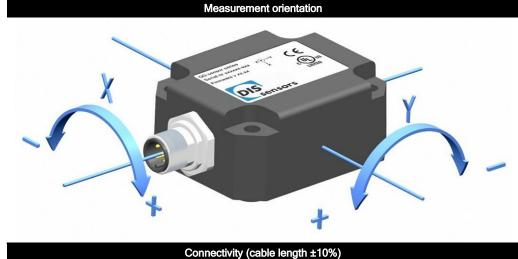
M12 male 5p A-coding connector (Brass Nickel coated, contacts copper alloy) + Supply voltage Output Y Gnd Pin 1: Pin 2: Pin 3: Pin 4: Output X Zero adjustment input Pin 5: Male
