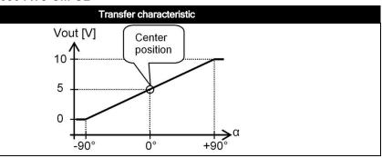
Default 0°: horizontal (label upwards), no acceleration applied.
