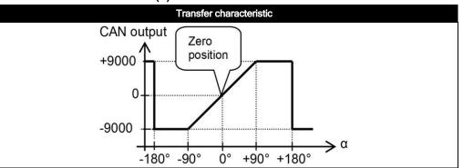
Default 0°: horizontal (label upwards), no acceleration applied. To eliminate mounting offsets the sensor can be zero-ed within ±5° tilt (by the CAN object dictionary)
