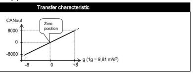
The default 0 g position is when the sensor is mounted horizontal or vertical and no acceleration is applied. The axis parallel to earth gravity will indicate 1 g, the two horizontal axes will indicate 0 g. The two horizontal axes can be zeroed within ±5° tilt (by the CAN object dictionary) to eliminate mounting offsets.
