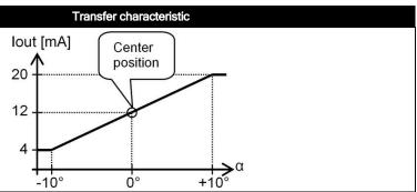
Default 0°: horizontal (label upwards), no acceleration applied.
