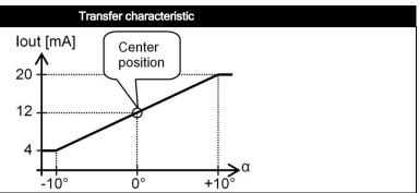
Default 0°: horizontal (label upwards), no acceleration applied.
