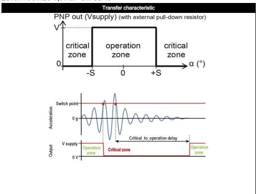
The default 0 g position is when the sensor is mounted in any position and no acceleration is applied.
