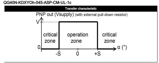
The default 0° position is when the sensor is mounted horizontally (round nose upwards) and no acceleration is applied.
