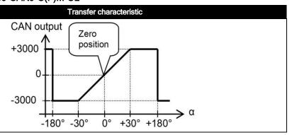
Default 0°: horizontal (label upwards), no acceleration applied. To eliminate mounting offsets the sensor can be zero-ed within ±5° tilt (by the CAN object dictionary)
