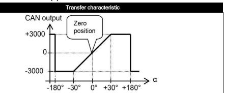
Default 0°: horizontal (label upwards), no acceleration applied. To eliminate mounting offsets the sensor can be centered within ±5° tilt (by the CAN object dictionary)
