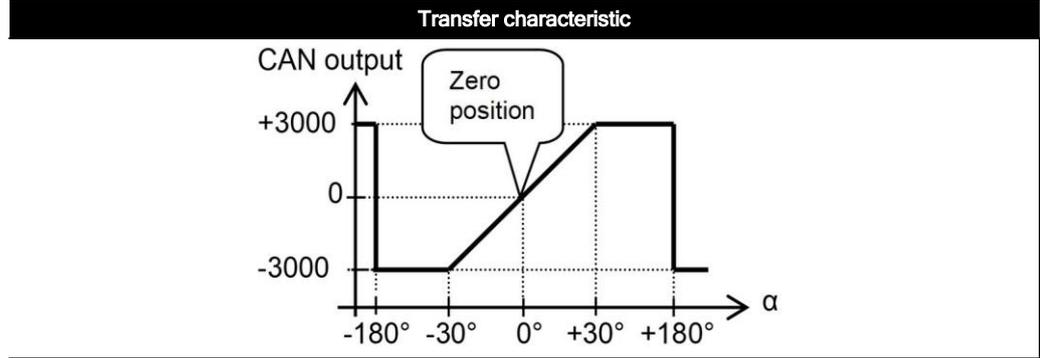
Default 0°: horizontal (label upwards), no acceleration applied. To eliminate mounting offsets the sensor can be zero-ed within ±5° tilt (by the CAN object dictionary)
