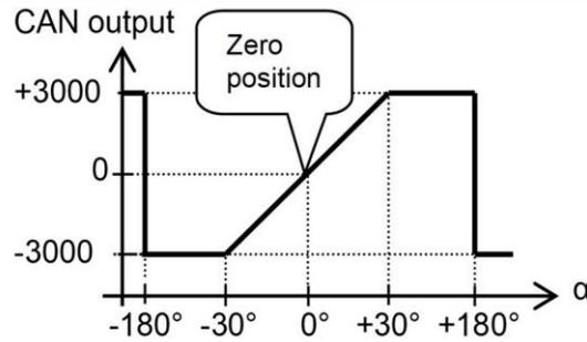
Default 0°: horizontal (label upwards), no acceleration applied. To eliminate mounting offsets the sensor can be zero-ed within  $\pm 5^\circ$  tilt (by the CAN object dictionary)
