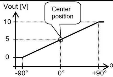
Default  $0^\circ$ : horizontal (label upwards), no acceleration applied.
