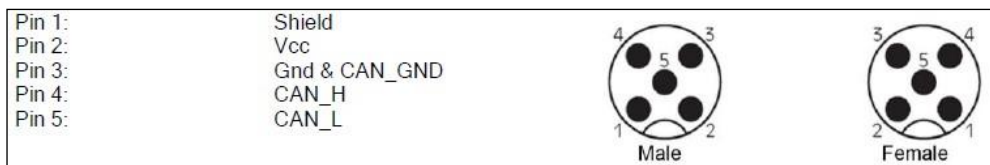
Figure 1: Layout CAN bus connector
