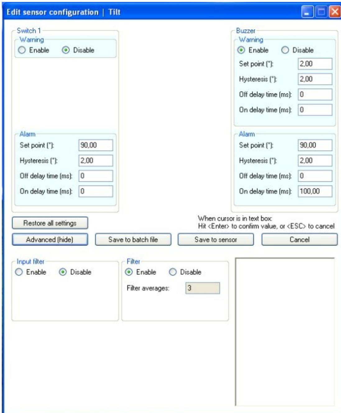
Configuring a Tilt sensor with 1 switching output and internal buzzer (advanced window shown)
