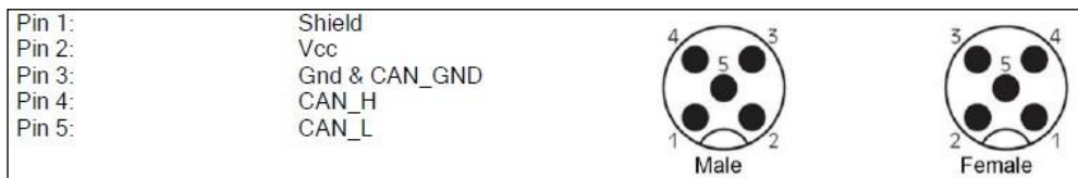
Figure 1: Layout CAN bus connector
