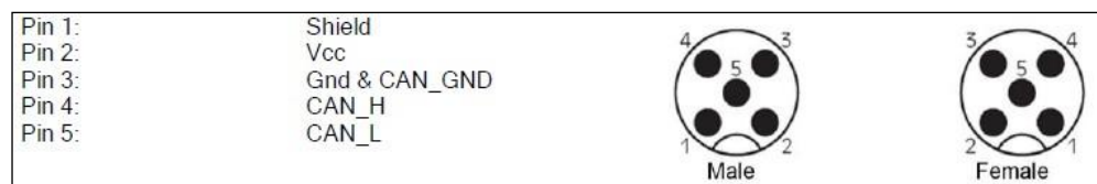
Figure 1: Layout CAN bus connector
