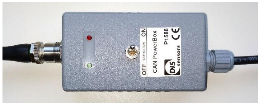
Figure 3 - CAN power box
