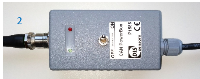
Figure 21 - CAN power box
