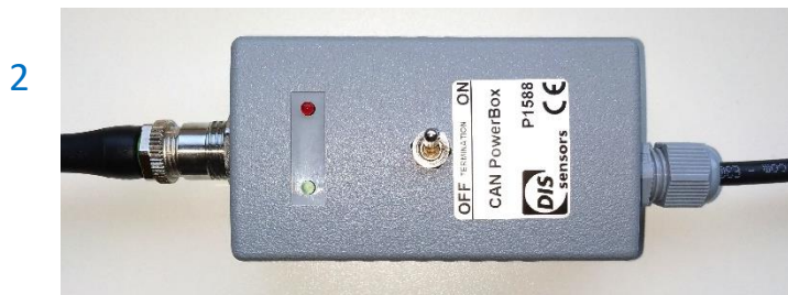
Figure 23 - CAN power box
