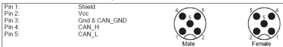
Figure 1: Layout CAN bus connector
