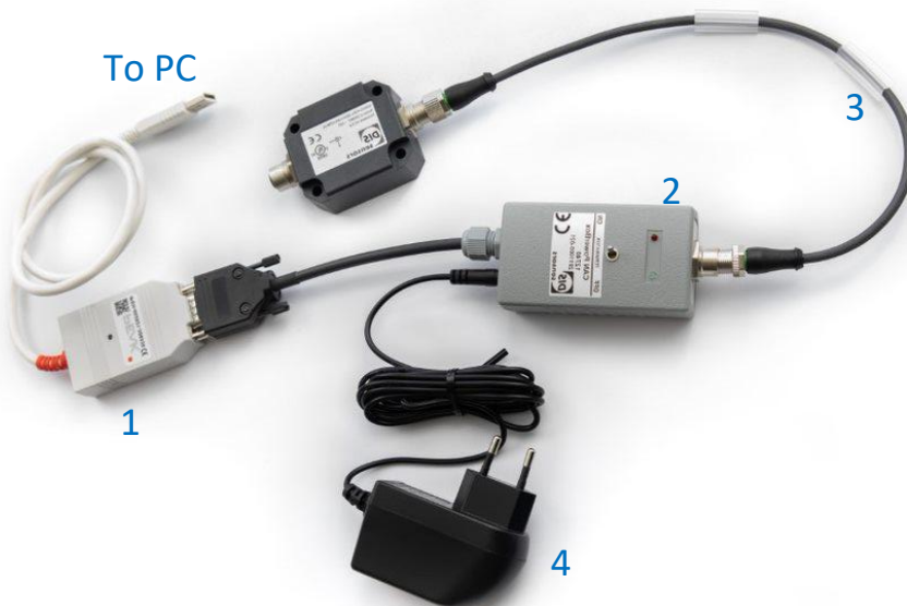
Figure 18 - Connection of DIS configurator set CAN
